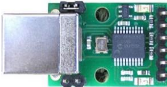
USB-ISS – Multifunctional communication module, mounted on each finger.
